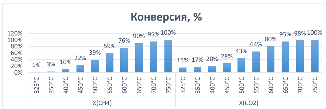
1-рasm. (\text{Ni}_2\text{O}_3)_x * (\text{Co}_2\text{O}_3)_y * (\text{ZrO}_2)_z * (\text{B}_2\text{O}_3)_k * \text{Me}/\text{Al}_2\text{O}_3 katalizatorida metanni bug'-karbonatli konversiyalashda SN 4 va SO 2 katalitik o'zga-rish darajasiga haroratning ta'siri (SN 4 :SO 2 =1:1; R=0,1 MPa; V 0 =1000 soat -1 )
