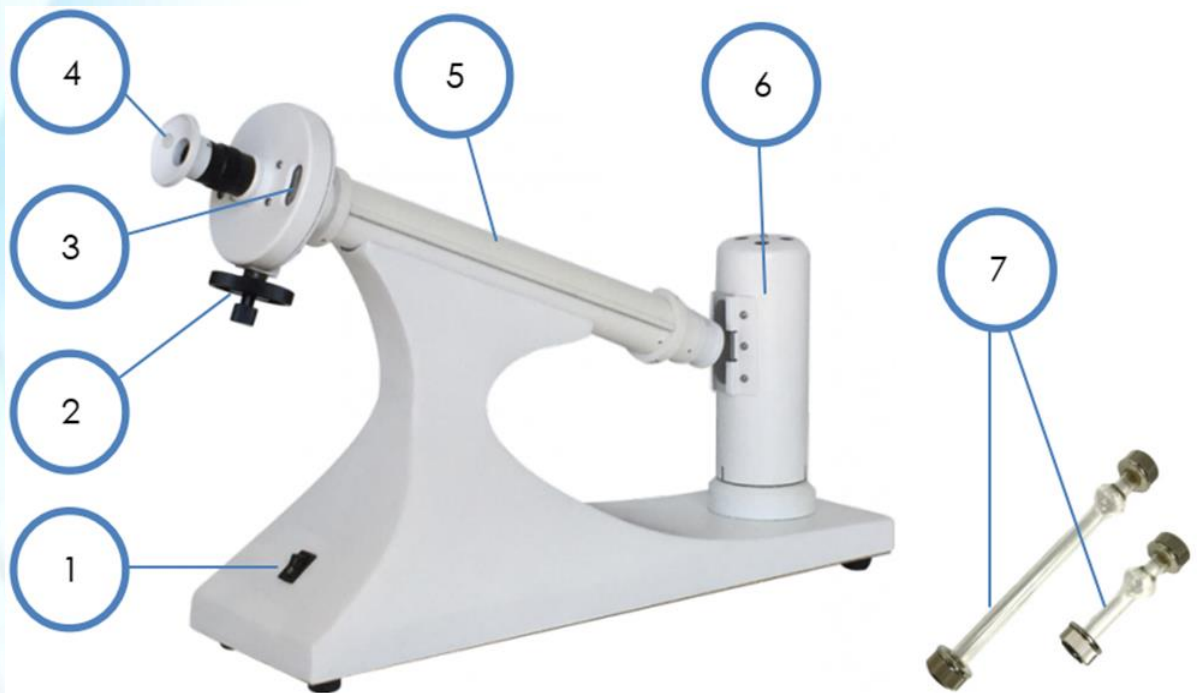
3-rasm. Polyarimetr. 1 - yoqish tugmasi; 2 - analizatorning burish vinti; 3 - asbob shkalasi; 4 - ko'rish trubkasini fokuslash muftasi; 5 - kyuvetalar uchun kamera; 6 - yorug'lik manbai; 7 - kyuvetalar.
