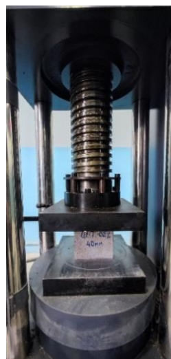
1-рasm. Beton kub na`munalarni sinov jarayoni
