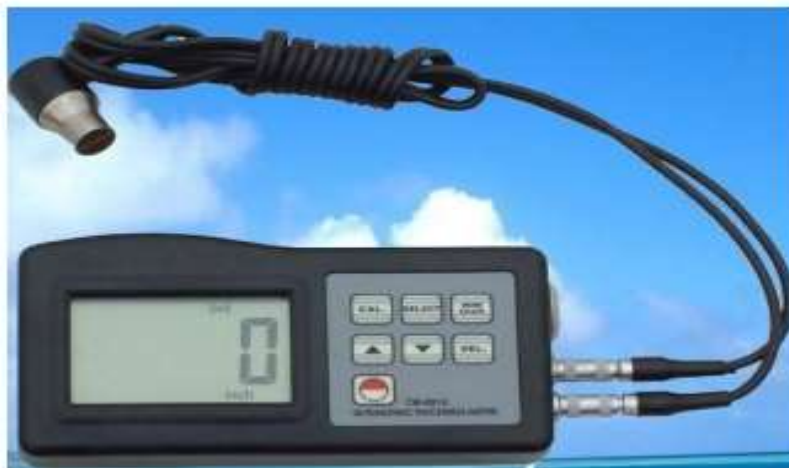
Figure 3. Ultrasonic thickness gauge MT 8812.
