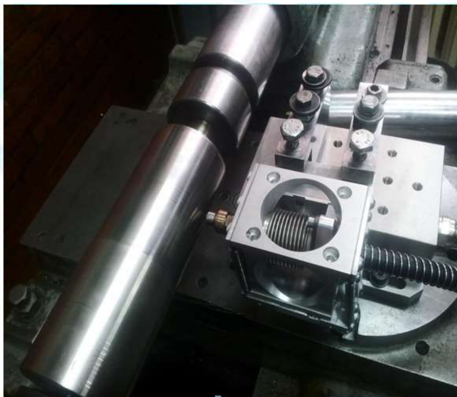
Rice. 4. Air spring mandrel installed on the machine with a receiver.
