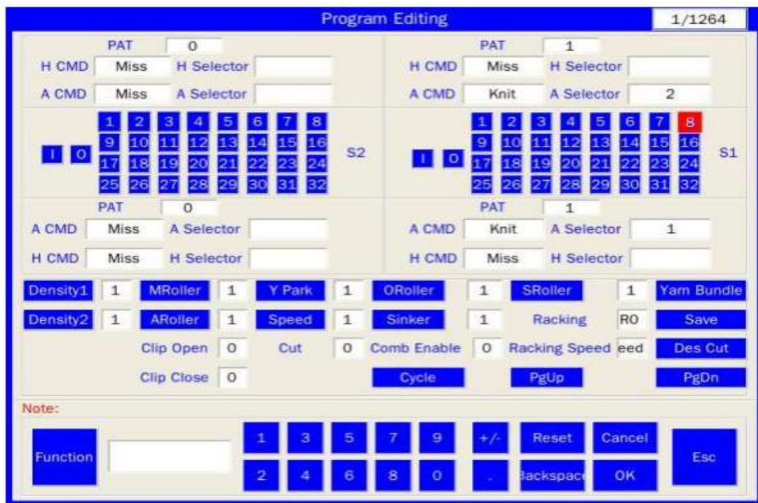
2-rasm. LONG XING yassi ignadonli trikotaj mashinasida dastur tahrirlash (Program Editing) interfeysi
